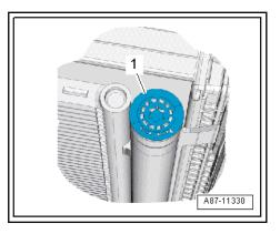
Moisten new seals with refrigerant oil before installing refrigerant line.
