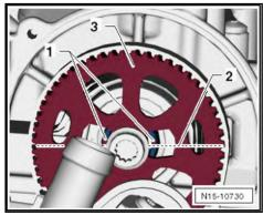
The centre-line of the holes close to hub of the gear -3- is slightly above the grooves.
