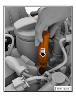
The "BDC" has been reached before the screwdriver starts moving back in opposite direction.
