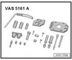
♦ Valve stem seal fitting tool -3365-
